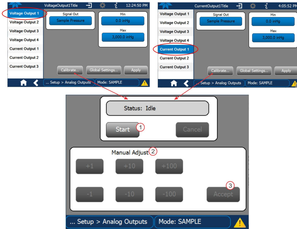
Figure 2-43. Analog Output Calibration, Voltage or Current
